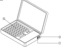
① Power Switch: Switch to ON to power on the charging case, and the LED will illuminate red. Switch to OFF to turn off the power, and the red LED will go off.
