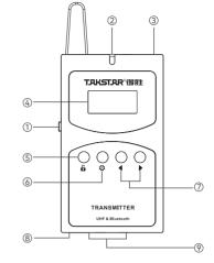
① Power Switch: Set to ON or OFF to power on/off the device respectively. (2) Indicator Light: Shows device status such as pairing, wireless playback pairing and battery level via different light colors and patterns.
